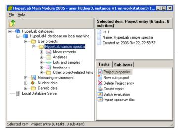
A new user project appears in the database browser tree. Open it, and click on *Measurements* node, then initiate the *Import spectrum files* task: simply click on it once in the Tasks window.
