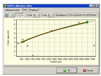
If large deviation found between the current calibration line (red line), and the suspected peaks' FWHM, then a miscalibrated FWHM may be suspected.
