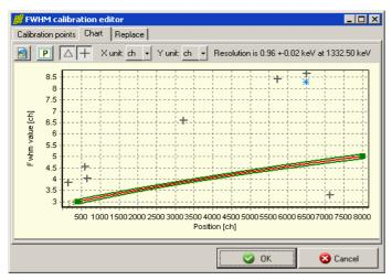
HyperLab's nonlinear spectrum deconvolution algorithm requires only a rough peak width (FWHM) calibration to start working. For exact peak positions, a valid energy calibration is also required.
